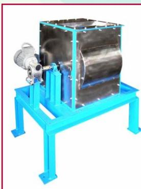
The drum separator can be used for material with small particle size (5 cm max.), where material is poured using a trough to a stainless steel drum that rotates around a fixed magnet inside the drum. The magnet catches magnetic metals and removes them behind a separating baffle.
