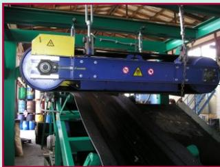
Cleaning of the magnet is solved on an overbelt principle, where the magnet is placed inside the conveyor, whose belt provides moving of metals out of the transport routes.
